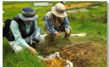
Drilling activity to make monitoring point for Radon and Mercury also for gas sampling, total there are 18 holes were dedicated for monitoring points (left).
